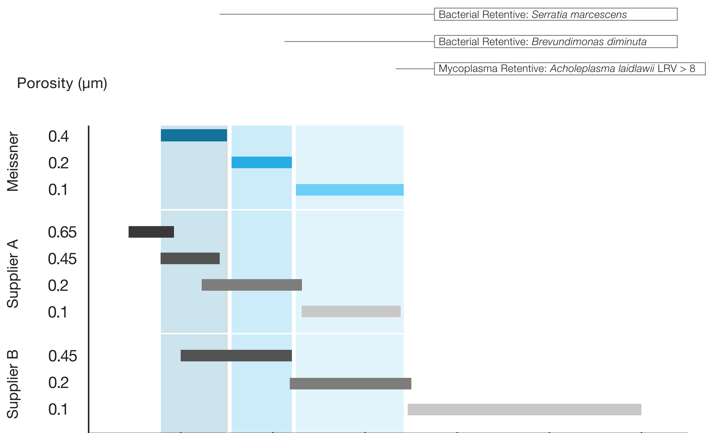
SeptraPor® filters' narrow bubble point ranges were established using industry-standard microbial retention assays, and have no overlap between pore sizes for improved process reproducibility. Supplier A has overlapping bubble point ranges which creates arbitrary pore size designations, while Supplier B has broad bubble point ranges that can lead to process variability over the entire acceptable spectrum.
