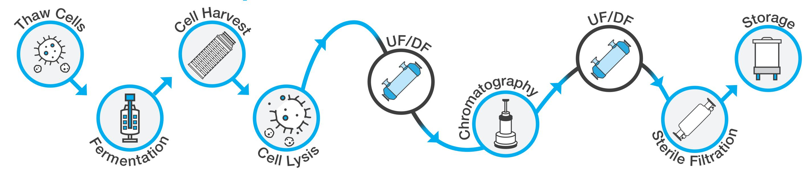
This generic pDNA manufacturing process diagram demonstrates that there are several critical UF/DF steps to ensure impurity removal and successful exchange of buffer for subsequent processing. Process intensification using SepraPor® UF hollow fiber filters in these manufacturing steps offer advantages, including minimized processing time, reduction in buffer volume requirements, and decreased effective filtration area (EFA) requirements.
