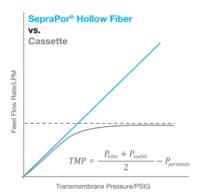
Plate-and-frame cassettes typically employ a tortuous flow path with restricted fluid entrance and exit openings. The restricted fluid inlet path results in a plateau in feed flow rate due to the accumulation of inlet back pressure. Alternatively, the hollow fiber form factor of SepraPor® UF filters allows for continuous increase in both pressure and feed flow rate, due to minimal fluid inlet restrictions.
