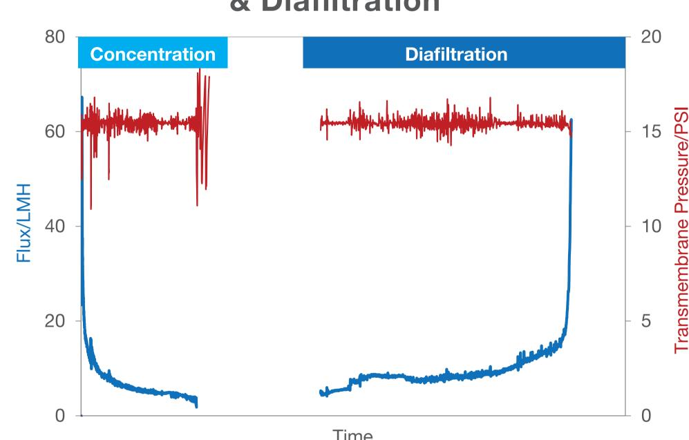
With transmembrane pressure (TMP) held constant, other relevant process parameters were monitored to evaluate the progress of the UF/DF process, such as flux, concentration factor, conductivity, and diafiltration volumes.
