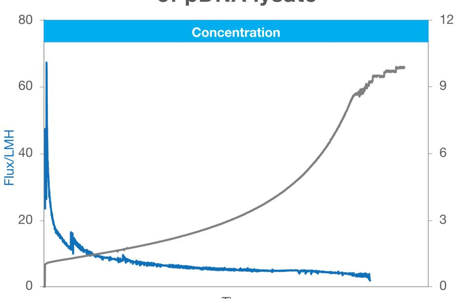
The initial concentration step proceeded until the target concentration factor of 10 was achieved. As expected, with constant TMP the flux dropped over time due to the increase in solution viscosity and membrane loading as the product was concentrated.
