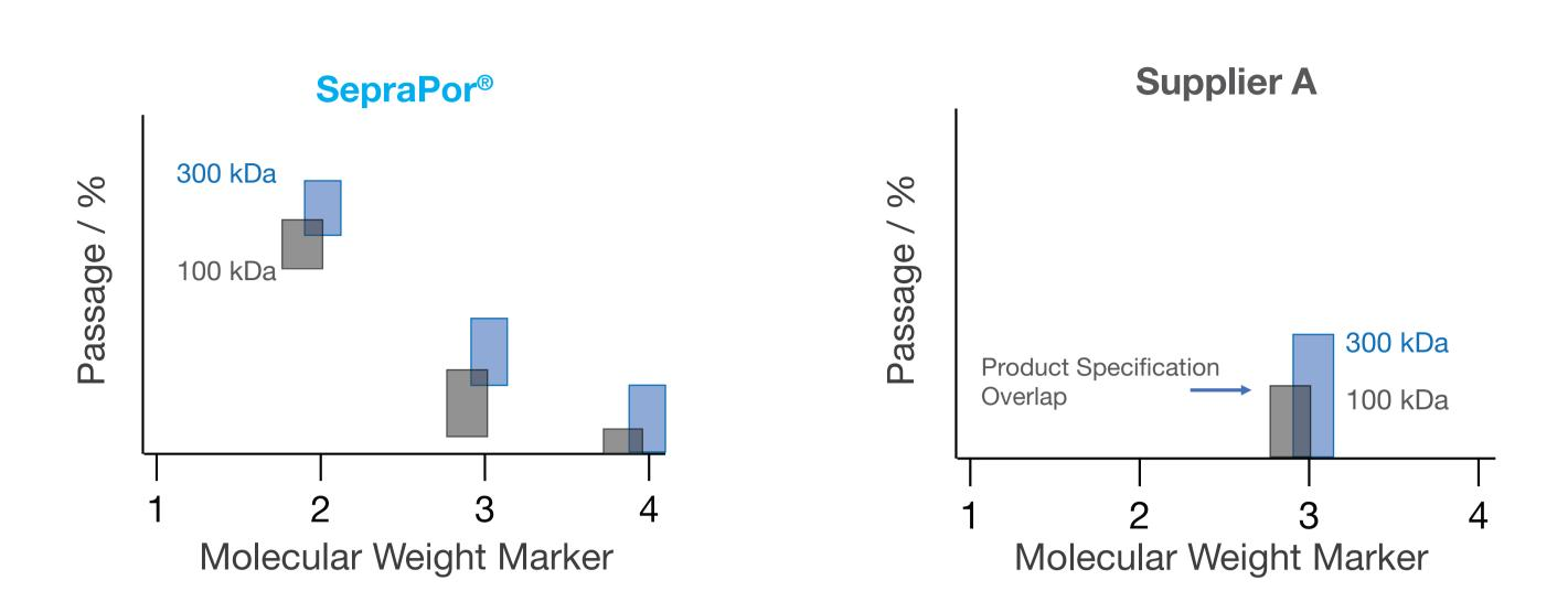
By using a minimum of three molecular weight (Mw) markers to characterize the molecular weight cut-off (MWCO) of a UF membrane, we are able to achieve well-defined MWCO membrane passages to ensure batch-to-batch consistency when performing process intensification in critical applications.
