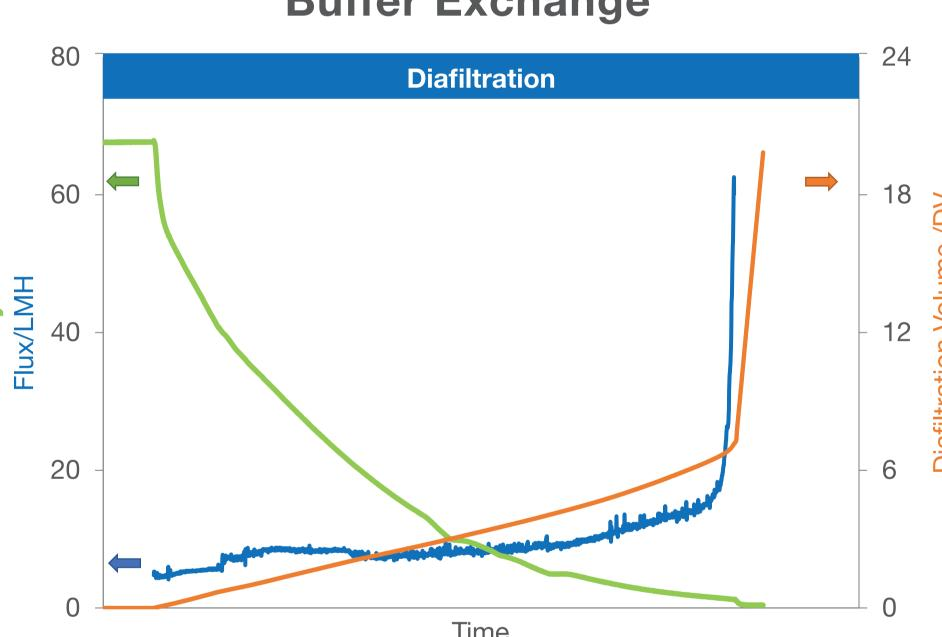
During the diafiltration step, fresh buffer was introduced into the concentrated product and tracked in diafiltration volumes, effectively increasing the total solution volume and diluting the product in the new buffer. This step was continued until the conductivity reached 0.5 mS/cm, indicating completion of the buffer exchange step.
