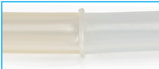
C-Flex® welds to M-Flex® using the same settings as required to weld C-Flex® 374.
