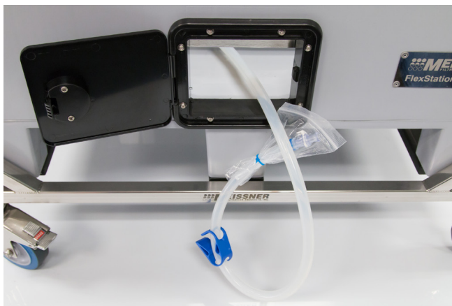
Tubing routed through hole in false bottom tray
