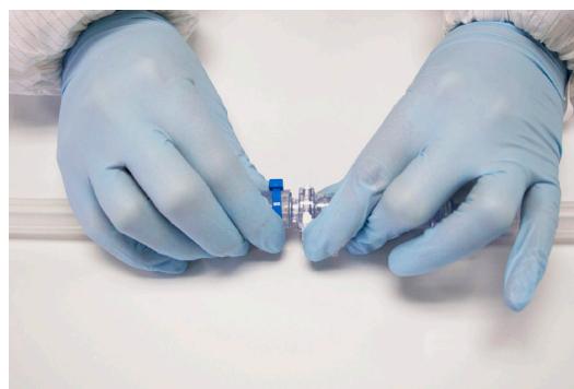
To disconnect, ensure that fluid flow is restricted accordingly and depress white latch on coupling body to pull coupling insert out.
