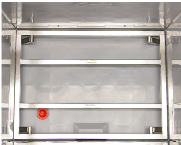
False bottom rack in place
