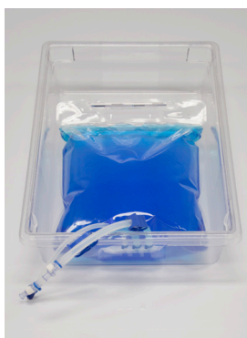
2D end-ported biocontainer in angled pillow position
